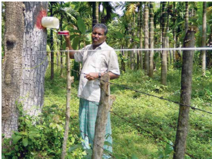
Trip alarm installed along the forest-farm boundary warns the villagers if elephants enter the field
